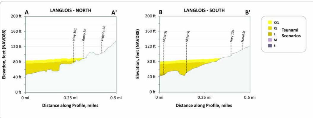
Figure 6: These profiles depict the expected maximum tsunami wave elevation for the five "tsunami T-shirt scenarios" along lines A-A' and B-B'. The tsunami scenarios are modeled to occur at high tide and to account for local subsidence or uplift of the ground surface.
